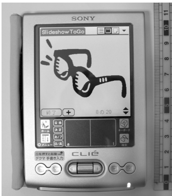
Fig. 1 A handy PDA with a square (55 × 55 mm), back-lighted LCD is used to display the objects during the naming task.
